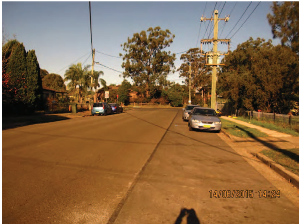
Octavia Street -Conveys major overland flows during heavy rain.
